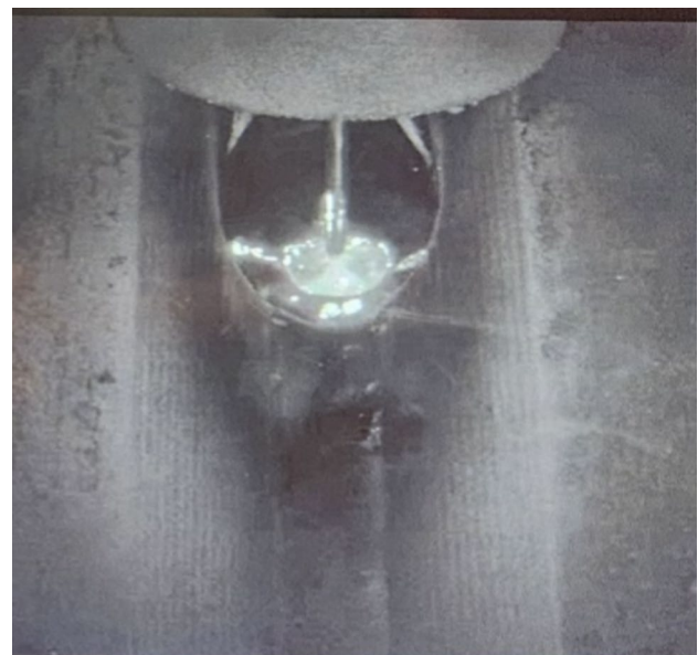
Fig. 5 Image taken with the welding camera from GMAW on a groove weld used in this work
