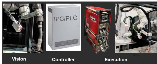
Fig. 4 A solution pipeline for perception and cognition of welders in robots
