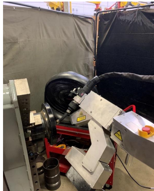
Figure 1 Collaborative spool welding robot used for video recording.
