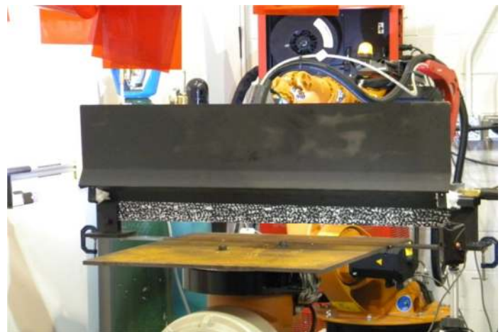
Figure 2 KUKA robot and Fronius welding units during welding. A metallic shield prevents the intense light from arc comes to the cameras.
